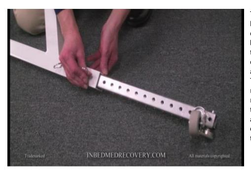
There are also horizontal legs that extend from the bases of the These triangles. can be extended for added stability. These may be removed and rotated 90 degrees, then re-inserted to allow either wheels or feet to contact the floor.
