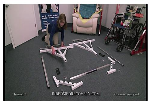
As can be seen in this photo, the triangular bases are identical. Two vertical bars are connected to the triangular bases and the two "shoulders". The shoulder pieces also connect to the horizontal bar. The horizontal bar, (which can be used a chin up or pull-up if bar done correctly) has the
